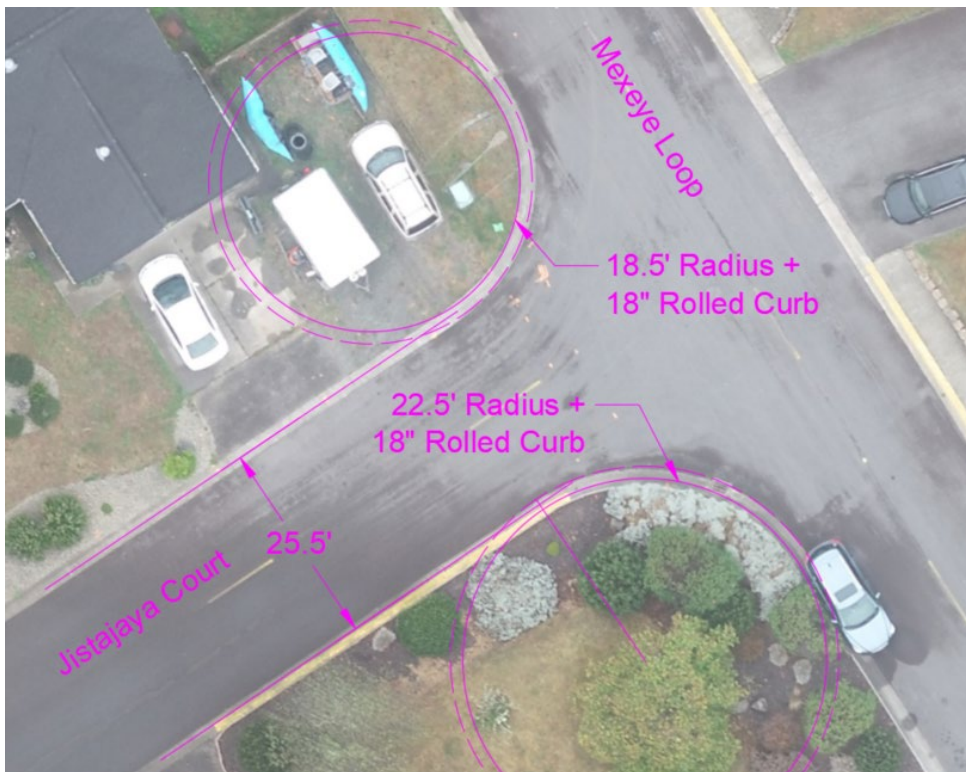
Jistajaya Court is 25.5' wide. The west curb is 18.5' radius and the east curb is 22.5' radius.
