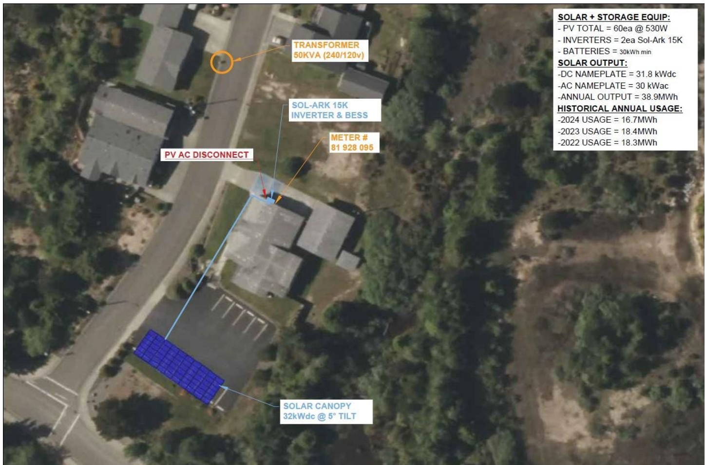
Figure 1 Proposed system development for CIHA Office bldg
