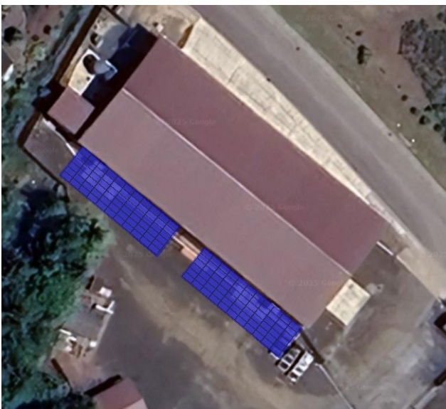
Fig 2.d - Concept for additional PV arrays. 35kWdc each
