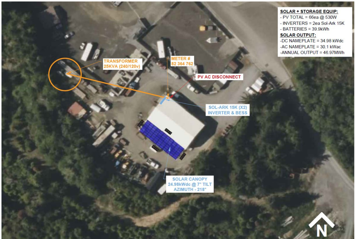
Figure 1 Proposed system for development at Maintenance Building
